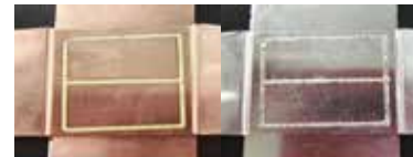
羽翼焊接 Wing assitant laser welding
